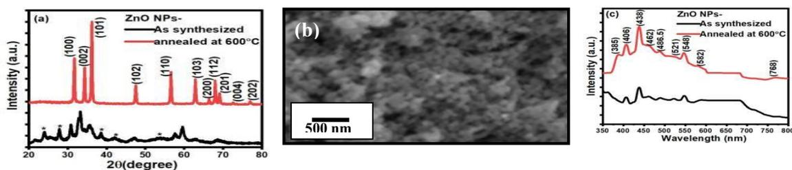
Fig 1. (a) XRD patterns (b) SEM image of ZnO NPs annealed at 600°C and (c) PL spectra of ZnO NPs
