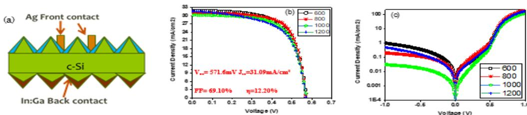
Fig: (a) A schematic of device structure of PEDOT:PSS/ $\mu$ T-Si solar cell (b) Illuminated J-V characteristics (insert best cell parameters ( $V_{oc}$ ,  $J_{sc}$ , FF, eff.) and (c) Dark J-V characteristics.
