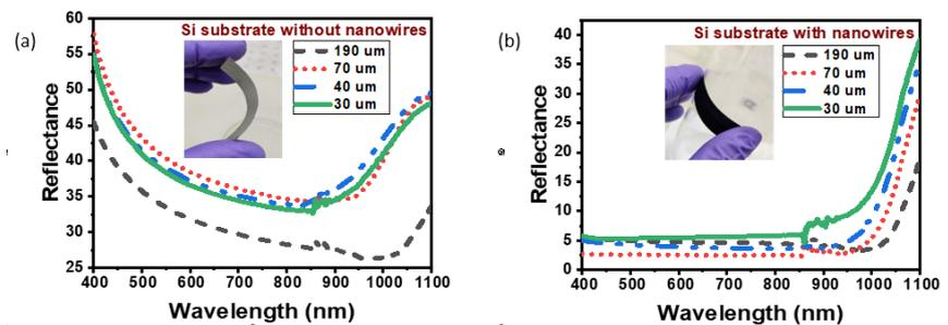
Fig: Reflectance curves for Si substrate (a) without nanowires and (b) with nanowires
