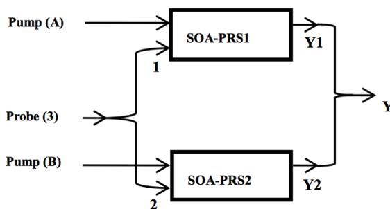
**Fig.1. Design of the Radix Converter**
