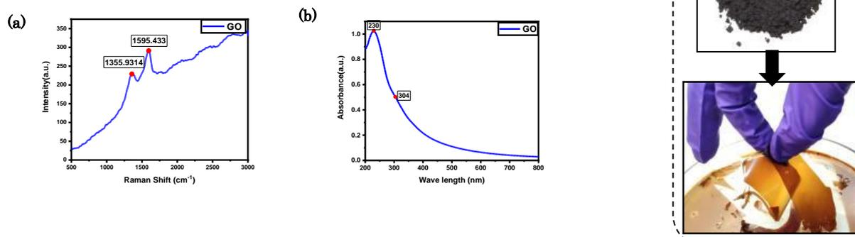
**Fig.1(a).** Representative Raman spectrum and, (b) UV-Vis spectrum of GO flakes, (c) Prepared GO flakes
