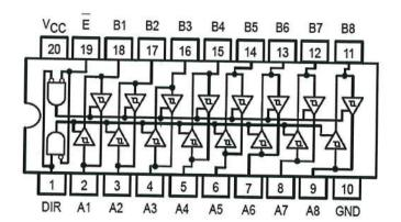
For the bidirectional buffer shown above, complete the operations (data flow direction) in following functional table for the given inputs.
