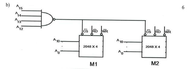
Identify the entire memory map (addresses) of the schematic shown above and explain the significance of the don't care address lines on the memory map.
