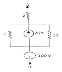
(b) Find the equivalent voltage source for the current source shown below. All resistances are in ohm. [5]
