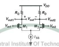
b) Draw the circuit diagram and its small signal equivalent of a differential amplifier with single ended output. Using small signal analysis, find the expression for ac voltage gain when a differential input is applied.
