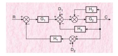
Calculate its transfer function  $\frac{C(s)}{R(s)}$  using Masson's gain formula. 10
