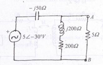
(c) What should be the value of  $R_L$  so that maximum power can be transferred from the source to load in the circuit given below?
