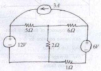
(b) Find voltage drop between terminals a and e for the following network.
