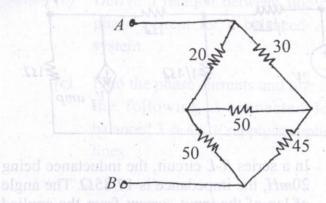
(b) In the circuit shown below, find I and voltage drop across  $R_I$ . 7
