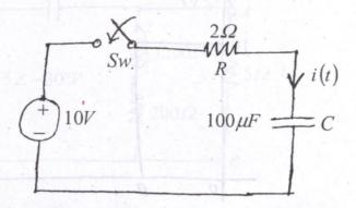
8. (a) A dc voltage of 100V is applied in the following circuit and the switch K is open. The switch K is closed at t = 0. Find the complete expression for the current 8
