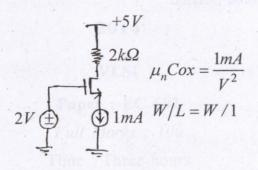
Find the value of  $V_{GS}$ ,  $V_{DS}$ ,  $g_m$  and  $r_0$
