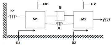
b) Draw the equivalent mechanical system of the figure shown below. Hence write the set of equilibrium equations and obtain electrical analogous circuits using F-V analogy and F-I analogy. (10)
