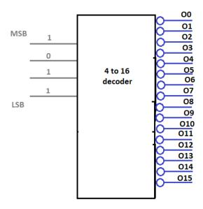
Specify the output line of the 4 to 16decoder that goes low if the input to the decoder is 1011 as shown in the figure.
