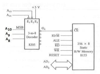
Identify the memory address range of the above interfacing. Also, mention the foldback /mirror memory ranges.
