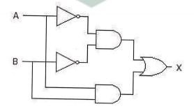
For the logic circuit diagram above, write its output expression and find out the truth table.
