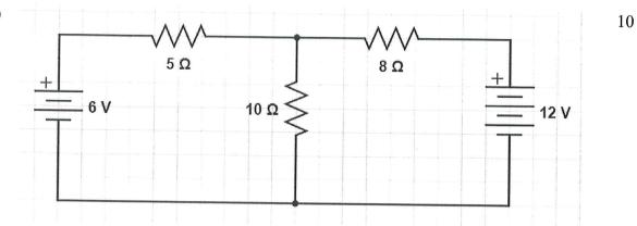
By using Superposition Theorem, find the current in resistance 10  $\Omega$  shown in Figure above.
