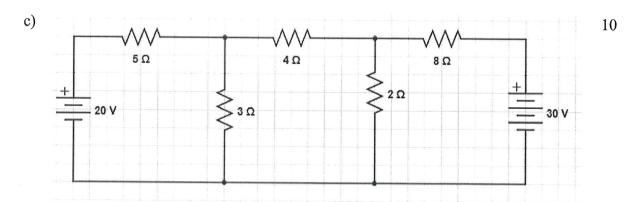
Find the current flowing through the  $4\Omega$  resistance using Maxwell's Loop Current Method.
