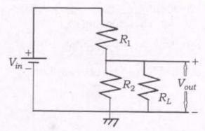
Determine the value of  $V_{out}$  when  $R_1 = 3k\Omega$ ,  $R_2 = 2k\Omega$ ,  $R_L = 1k\Omega$  and (ii)  $V_{in} = 5$  volts.
