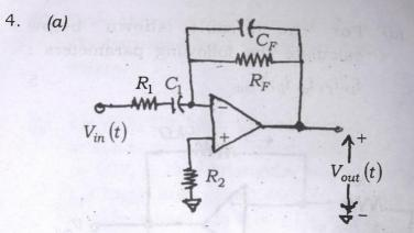
Derive the transfer function of the circuit shown above. Draw the magnitude response and derive the expression for the cut-off frequencies. What are the different applications of this circuit for various frequency ranges? 5+2+6+2
