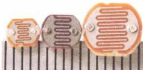
Figure 4: Three photoresistors with scale in mm
